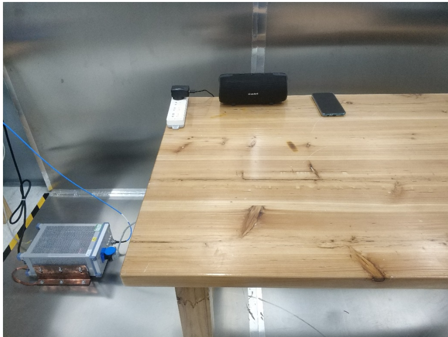
Photograph 3: Set-up for Conducted Emission on AC Mains
