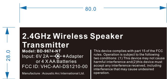
Transmitter rating label Size: 80x28mm Black background, white front, cover matte film+ back glue. Unit: mm Scale 1:1
