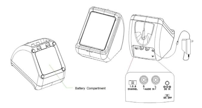
Turn the switch to On and the LED of transmitter will light up in Green. When the audio cable connection is finished and turn on the audio source, the LED will turn from Green to Blue.
