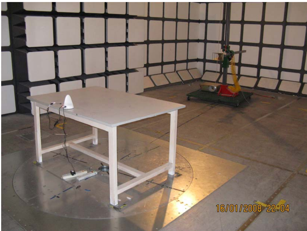
Radiated Emission - Rear View (30 -1000 MHz)
