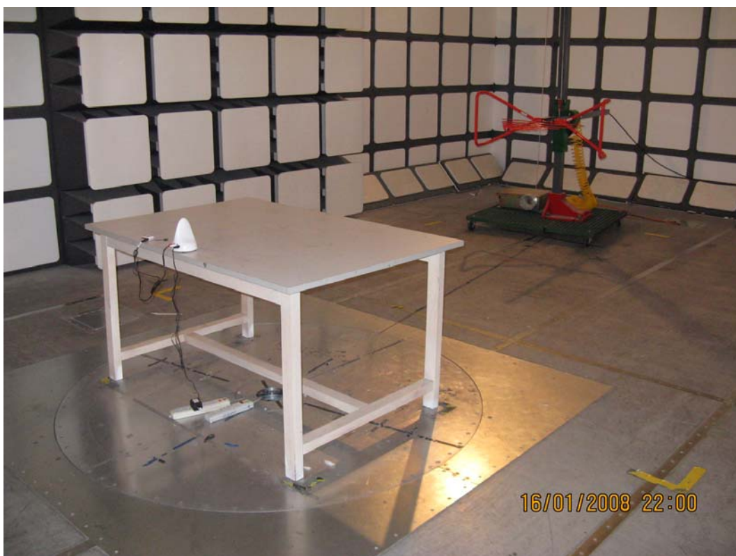
Radiated Emission - Rear View (Above 1 GHz)
