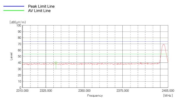
AV Detector: RBW: 1 MHz, VBW: 10 Hz (2 310 MHz - 2 390 MHz), Worst case (Low, Vertical)
