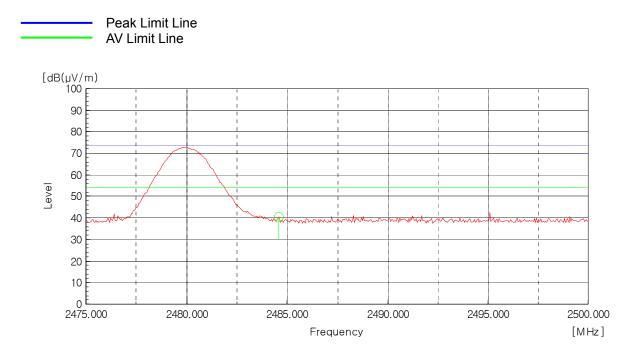
AV Detector: RBW: 1 MHz, VBW: 10 Hz (2 483.5 MHz - 2 500.0 MHz), Worst case (High, Vertical)
