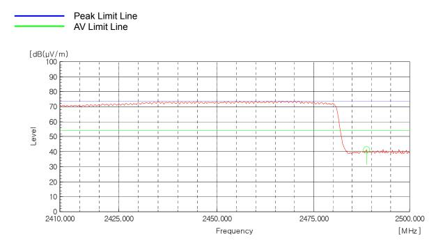
AV Detector: RBW: 1 MHz, VBW: 10 Hz (2 483.5 MHz - 2 500.0 MHz), Worst case (High, Vertical)
