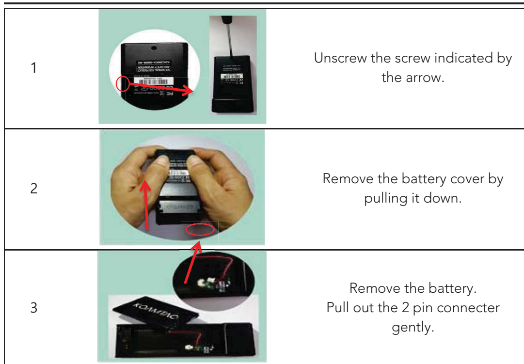
Figure 15 - Replacing a Battery
