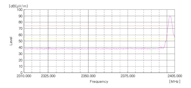
AV Detector: RBW: 1 MHz, VBW: 10 Hz (2 310 MHz - 2 405 MHz), Worst case (Low, Vertical)
