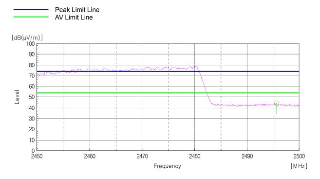
AV Detector: RBW: 1 MHz, VBW: 10 Hz (2 450.0 MHz - 2 500.0 MHz), Worst case (High, Vertical)
