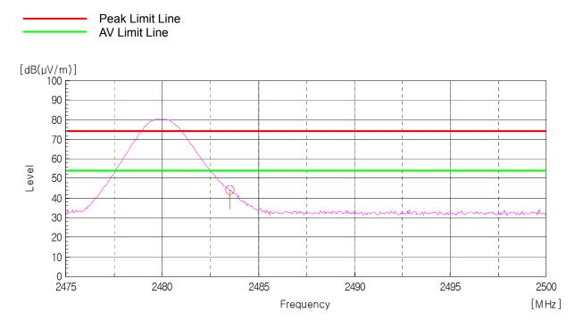
AV Detector: RBW: 1 MHz, VBW: 10 Hz (2 475.0 MHz - 2 500.0 MHz), Worst case (High, Vertical)
