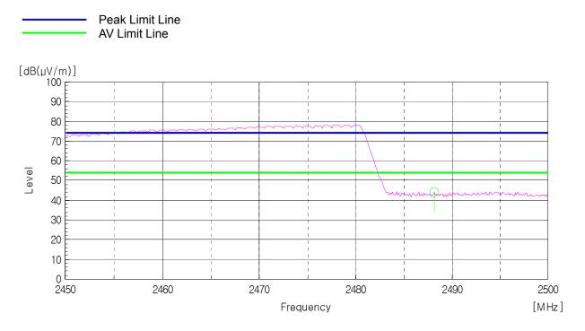
AV Detector: RBW: 1 MHz, VBW: 10 Hz (2 450.0 MHz - 2 500.0 MHz), Worst case (High, Vertical)
