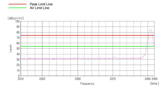
AV Detector: RBW: 1 MHz, VBW: 10 Hz (2 310 MHz - 2 405 MHz), Worst case (Low, Vertical)
