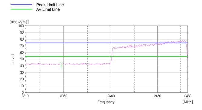
AV Detector: RBW: 1 MHz, VBW: 10 Hz (2 310 MHz - 2 483 MHz), Worst case (Low, Vertical)
