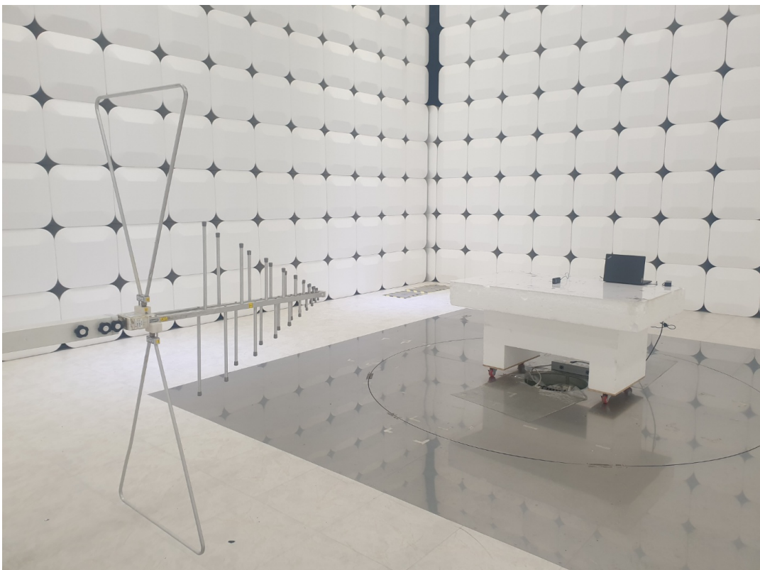
Radiated emission test (30 MHz to 1 GHz)
