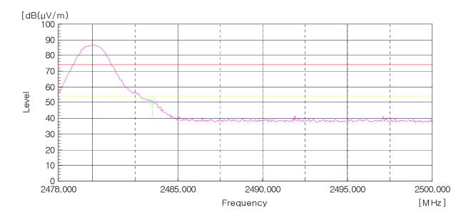
AV Detector: RBW: 1MHz, VBW: 10 Hz (2 478.0 MHz - 2 500.0 MHz), Worst case (High, Vertical)
