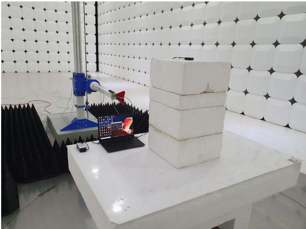
Radiated emission test (7 GHz to 18 GHz)
