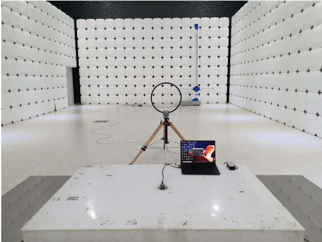
Radiated emission test (9 kHz to 30 MHz)
