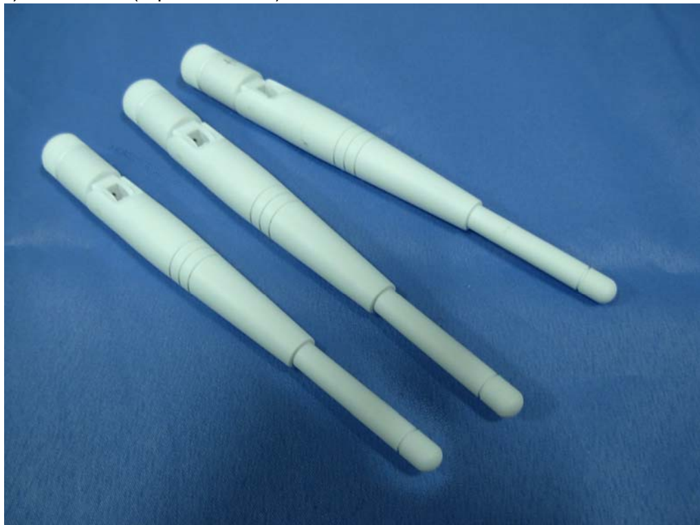
(26) EUT Photo (Dipole Antenna)
