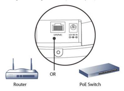
Connect VigorAP to PoE switch (via LAN port) with Ethernet cable. For connecting with PoE switch, do not connect the power adapter. VigorAP will get the power from the switch directly.
