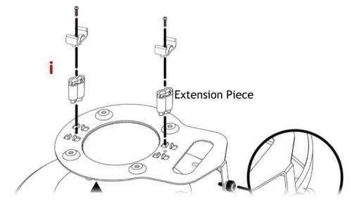
6. Attach the T-Rail brackets to the ceiling frame.
