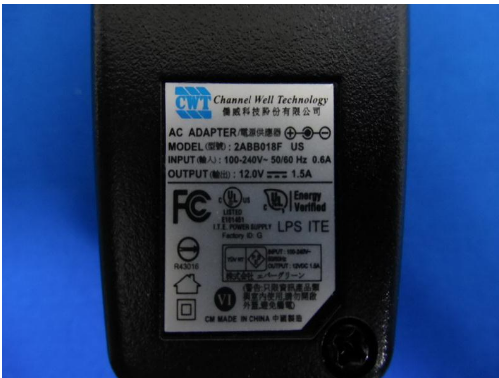
EUT - AC Adaptor Label (model: 2ABB018F US)
