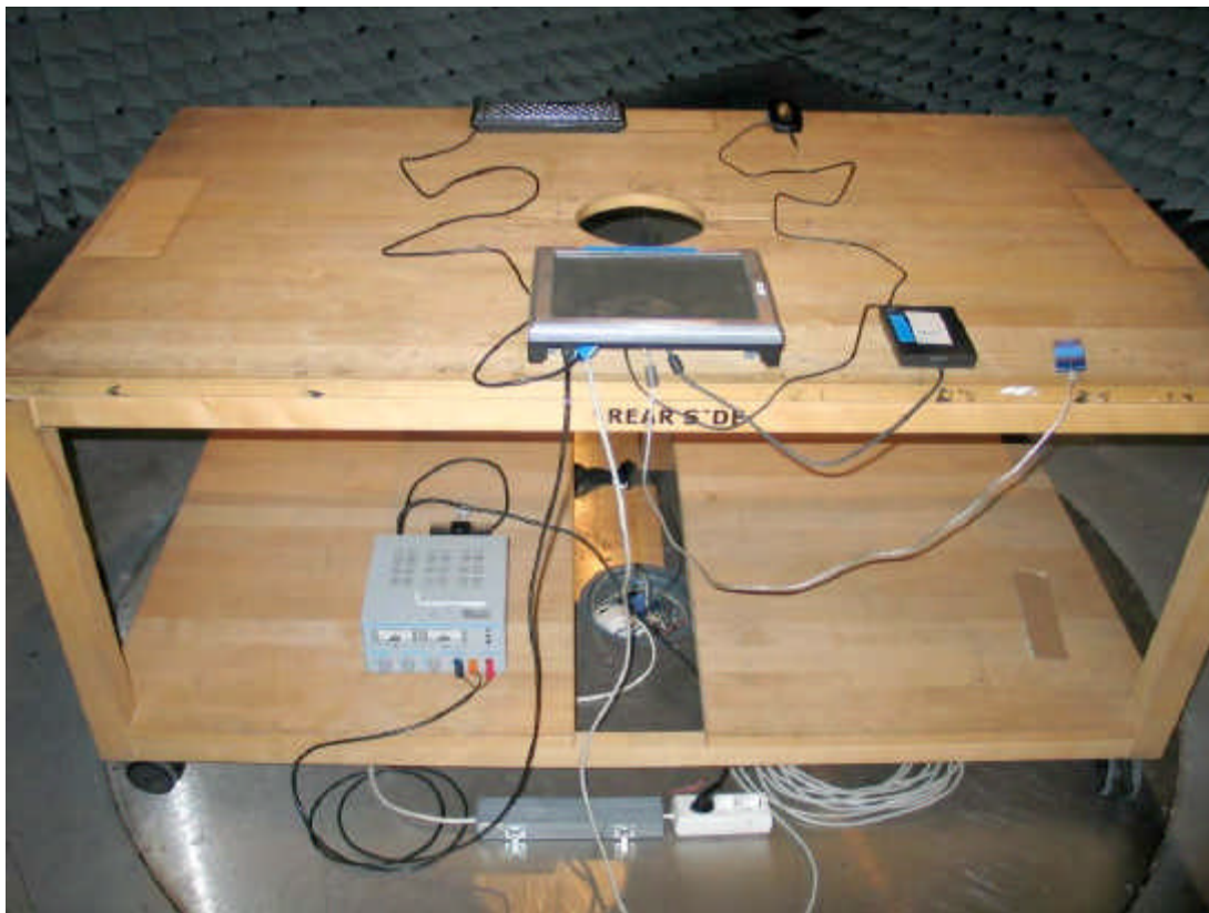
Photo 2: Test setup for radiated measurements below 1 GHz
