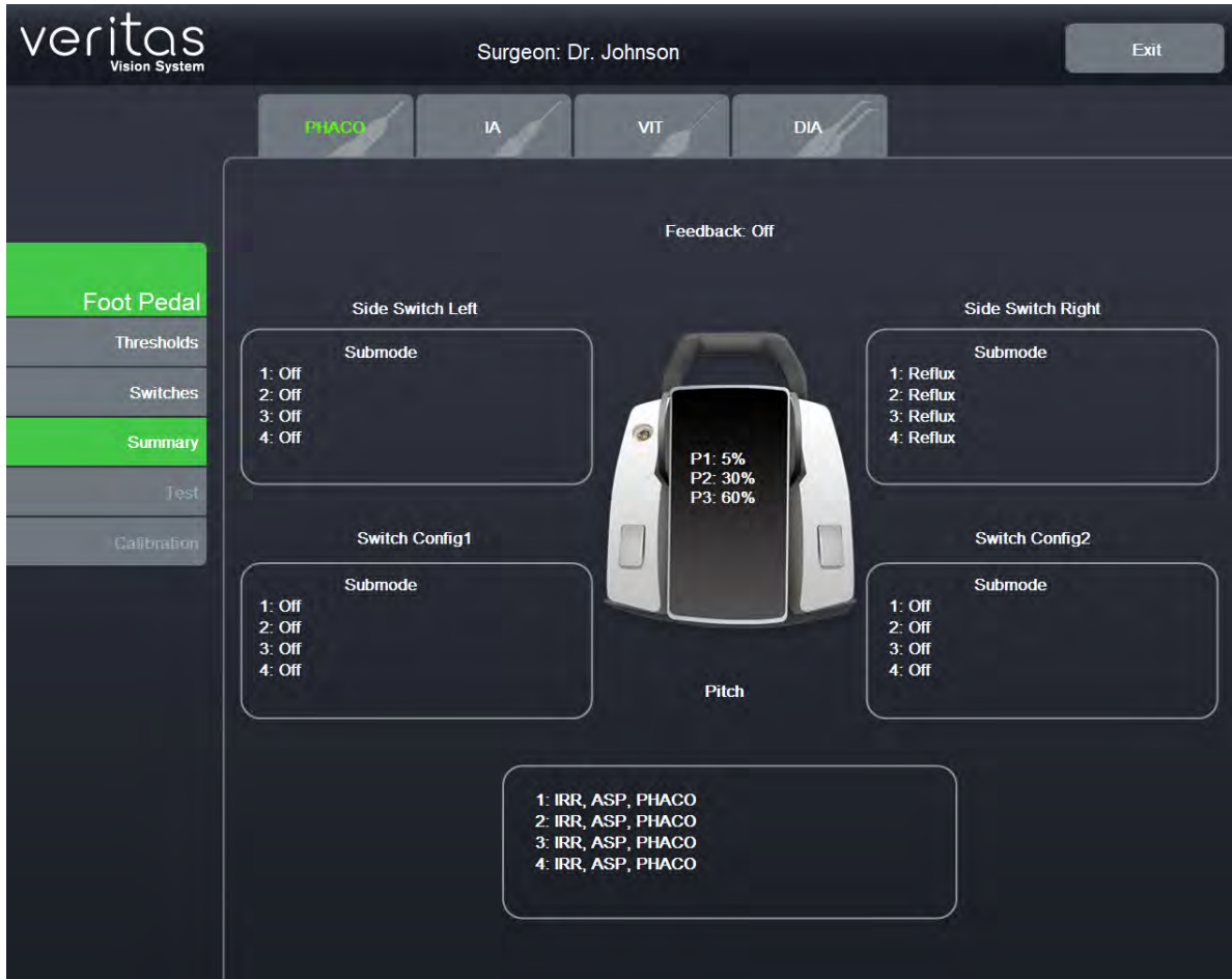
Figure 5-8 — Single Linear Foot Pedal Phaco Summary Screen
