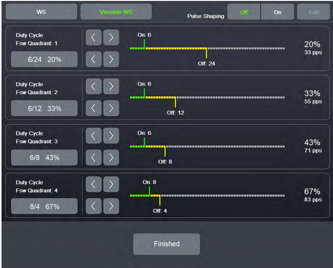
Figure 6-14 — Duty Cycles for Variable WS
