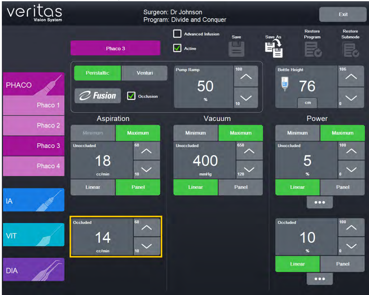
Figure 6-21 — Occlusion Aspiration Rate
