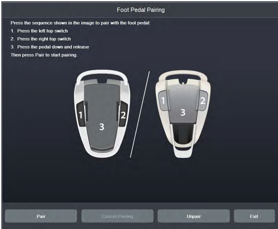
Figure 7-5 — VERITAS Foot Pedal and Advanced Linear Pedal Pairing Screen
