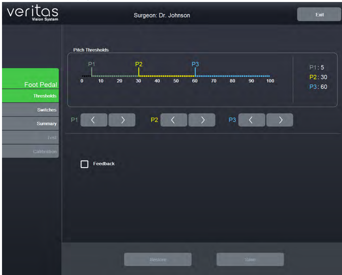
Figure 5-18 — VERITAS Foot Pedal Threshold Screen
