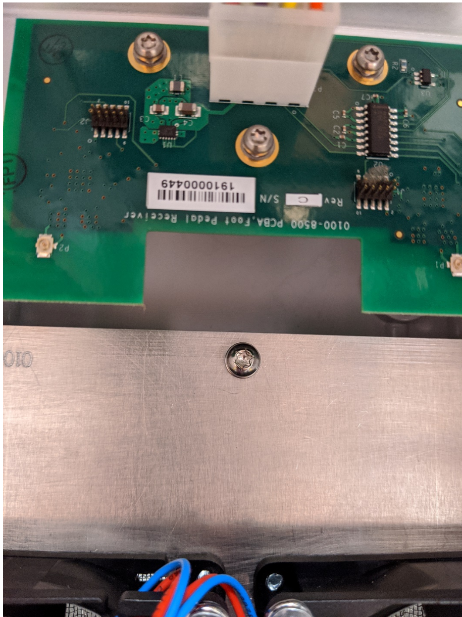
RF module for BLE Foot Pedal control mounted in main system
