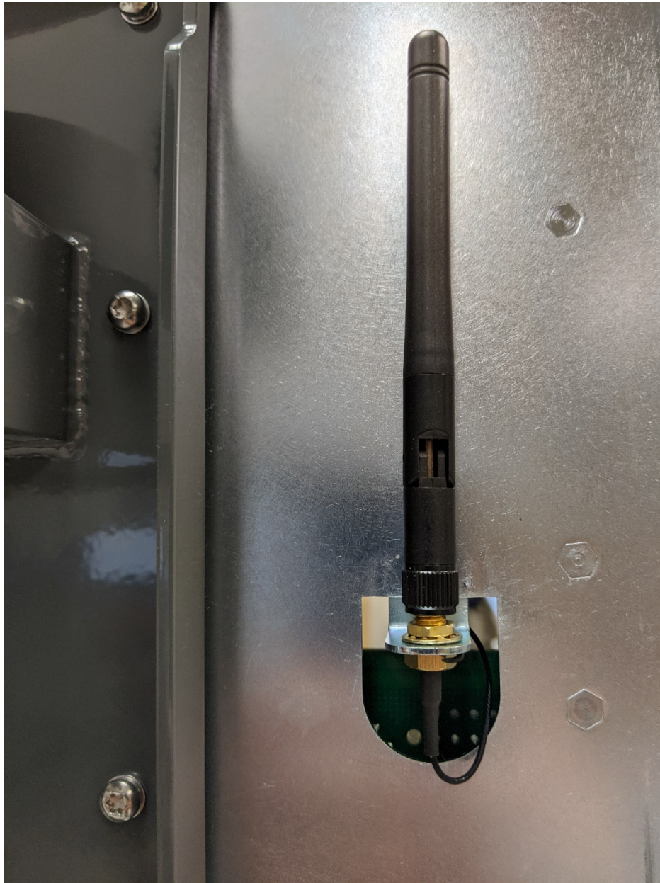
WiFi Antenna mounted in main system
