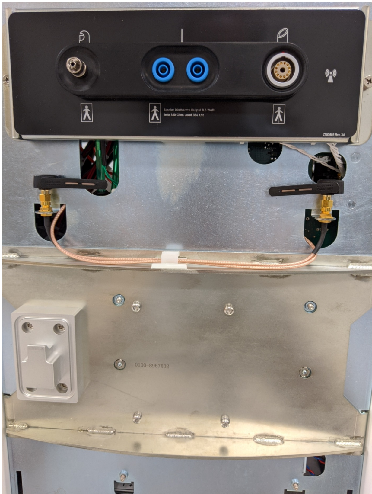
RF module for a Bluetooth Foot Pedal Control mounted in main system
