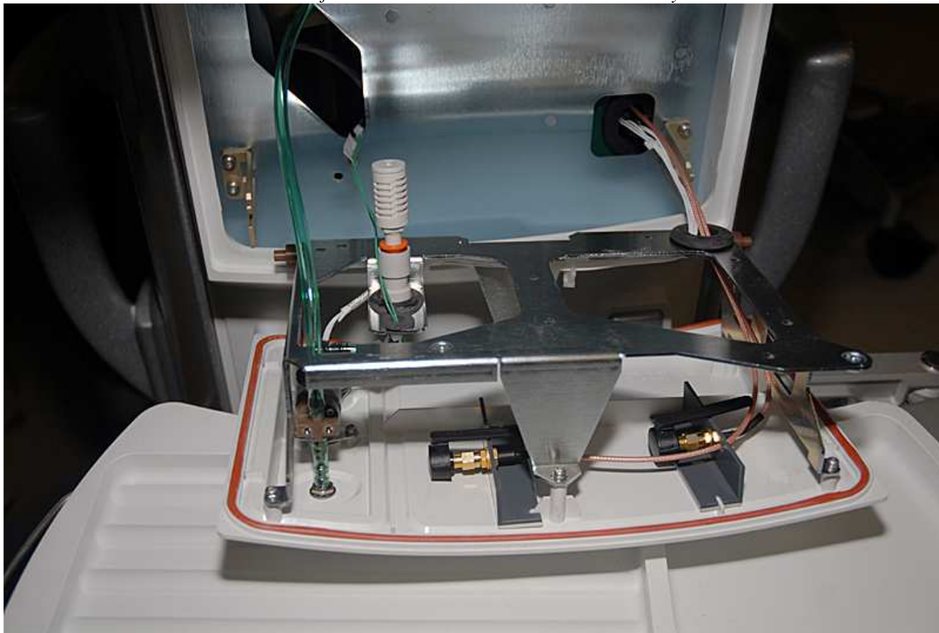
RF module for a Foot Pedal control mounted in main system
