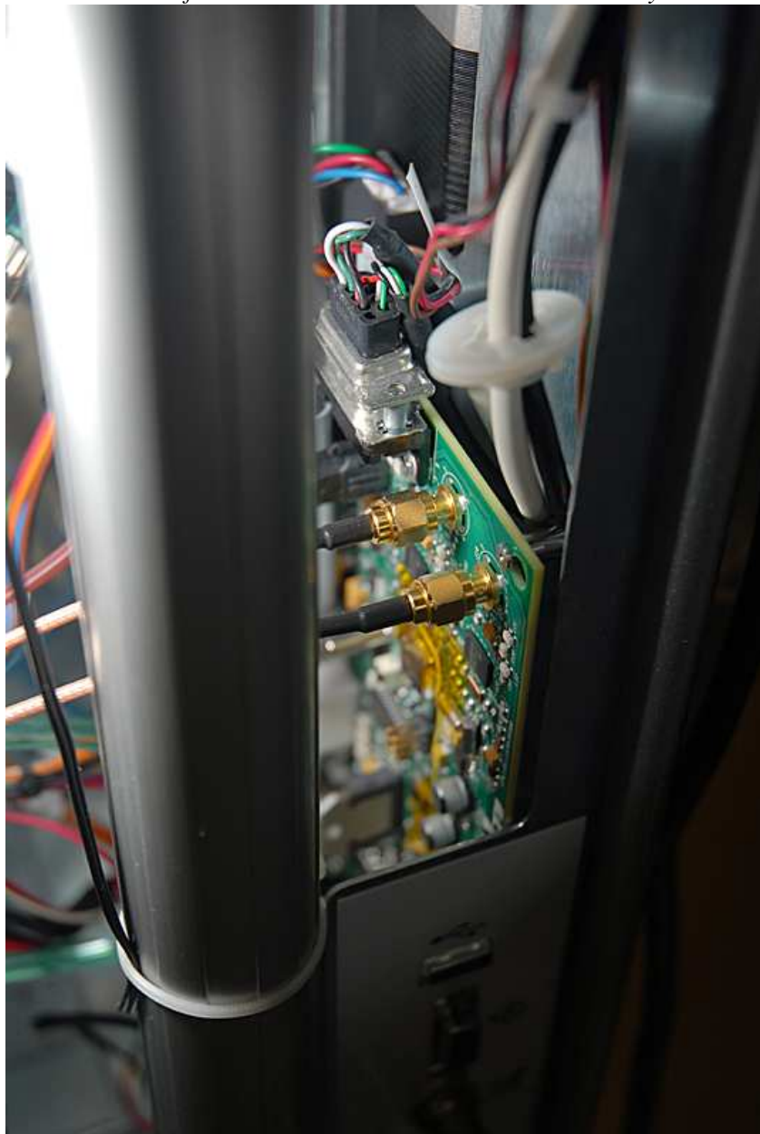
RF module for a Foot Pedal control mounted in main system
