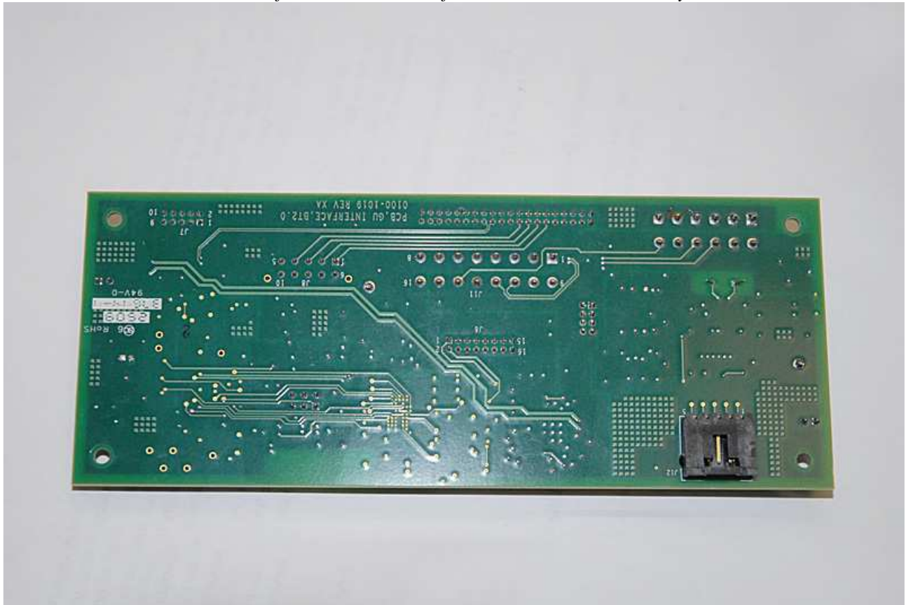
RF module for remote control of Monitor mounted in main system
