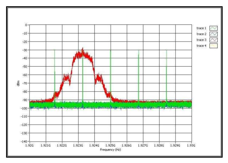
Comment1: Trace1 (green) is the interference on all 5 carriers. The level is Tu+UM+10dB. Comment2: Trace2 (blue) is interference on all 5 carriers. The level is TuR. Comment3: Trace3 (Red) is the EUT begins to transmit the beacon when interference is TuR.
