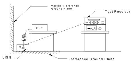
Test Set-Up 4
