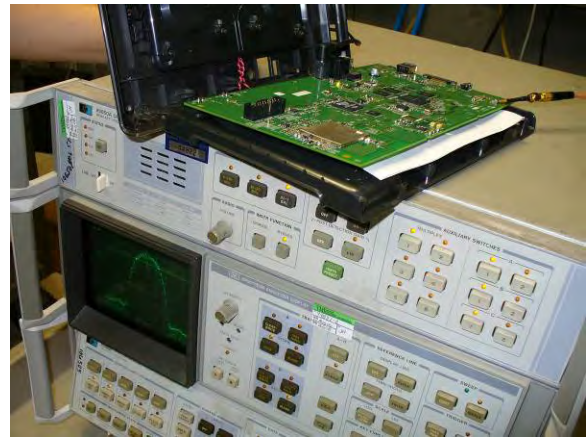
Photographs 5 and 6: Occupied Bandwidth and Power Spectral Density Setup
