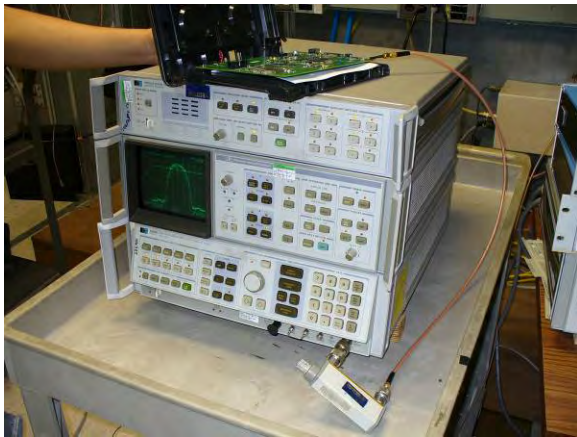
Photographs 5 and 6: Occupied Bandwidth and Power Spectral Density Setup
