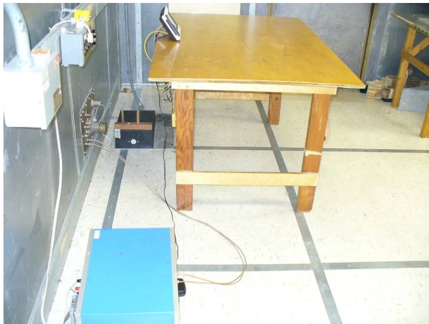
Photographs 1 & 2: Conducted Emission Setup
