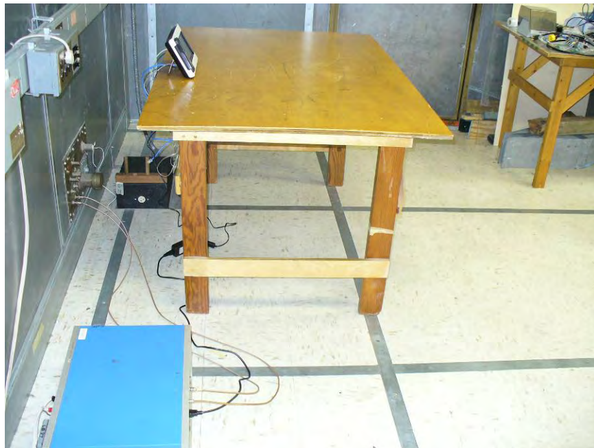
Photographs 1 & 2: Conducted Emission Setup
