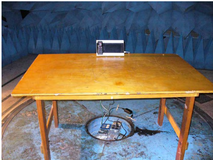
Photographs 3 & 4: Radiated Emission Setup
