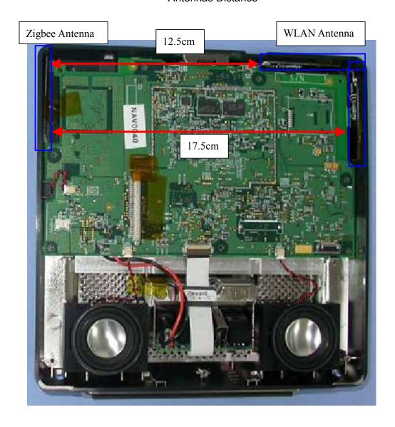
The antennas distance between Zigbee and WLAN is more than  $5\,\mathrm{cm}$ .
