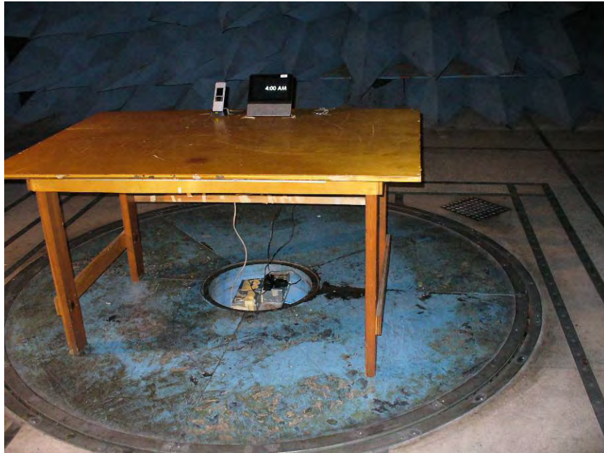
Photographs 3 & 4: Radiated Emission Setup
