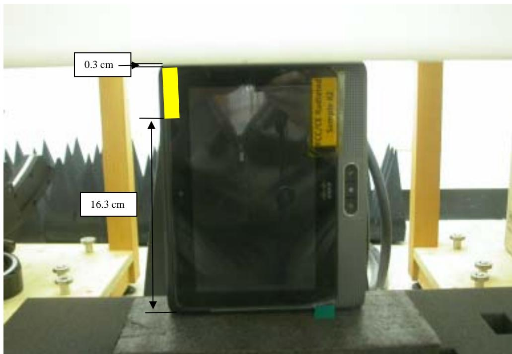
The EUT bottom to the ELI4 phantom distance is 0 mm.
