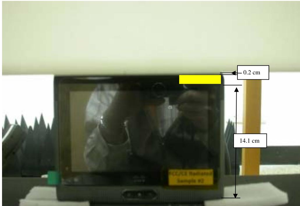
The EUT rear site to the ELI4 phantom distance is 0 mm..
