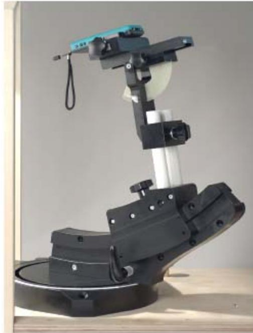
**Fig. 10 Device holder supplied by SPEAG**
