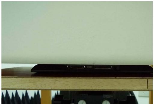
The EUT Bottom is in contact to the ELI4 phantom distance is 0 mm.
