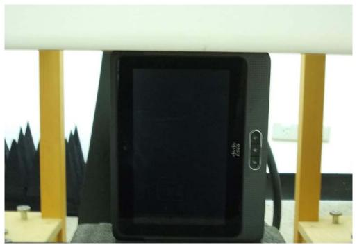
The EUT Secondary Portrait is in contact to the ELI4 phantom distance is 0 mm.
