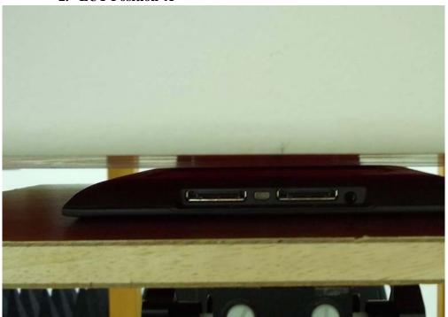
The EUT Bottom is in contact to the ELI4 phantom distance is 8 mm.
