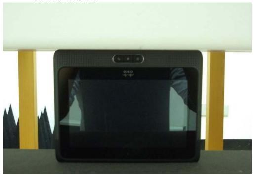
The EUT Secondary landscape is in contact to the ELI4 phantom distance is 0 mm.
