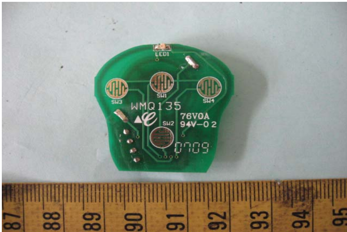
Component View of Main PCB
