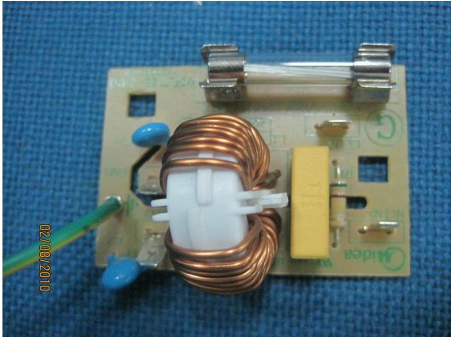
Power Filter Board- Top View
