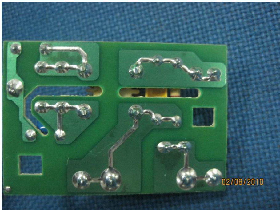
Power Filter Board -Bottom View
