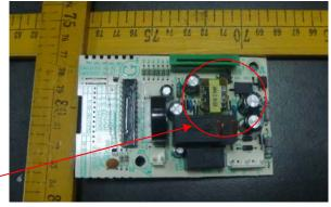
Changed linear power supply to switching power supply.
