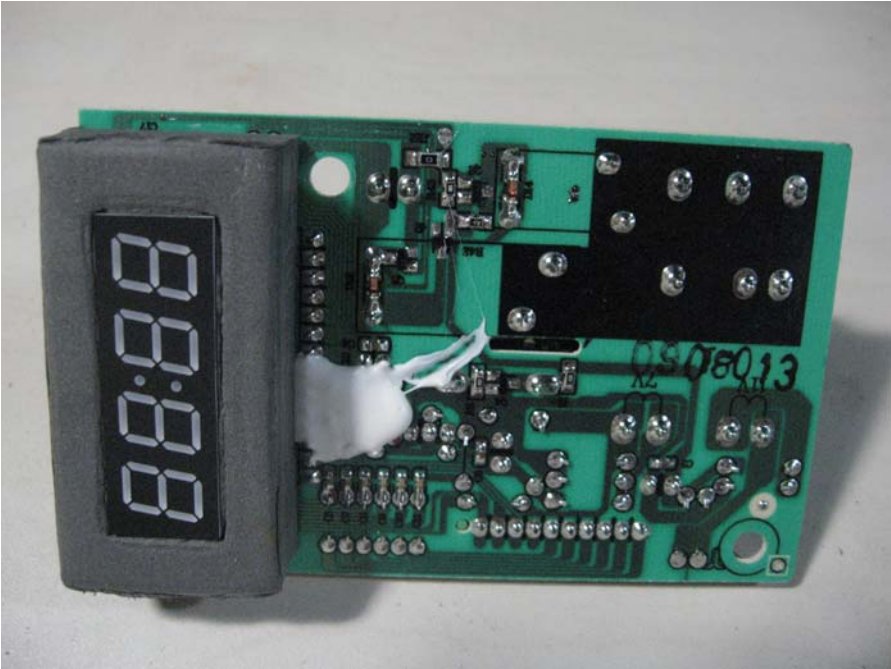
Control Board-Back View
