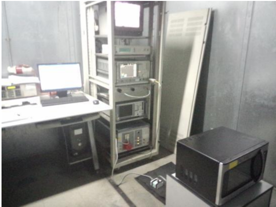
Conducted Emission Test Set-up
