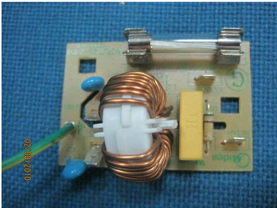
Power Filter Board Top View
