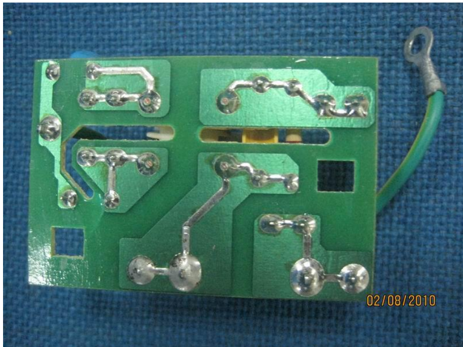
Power Filter Board Bottom View
