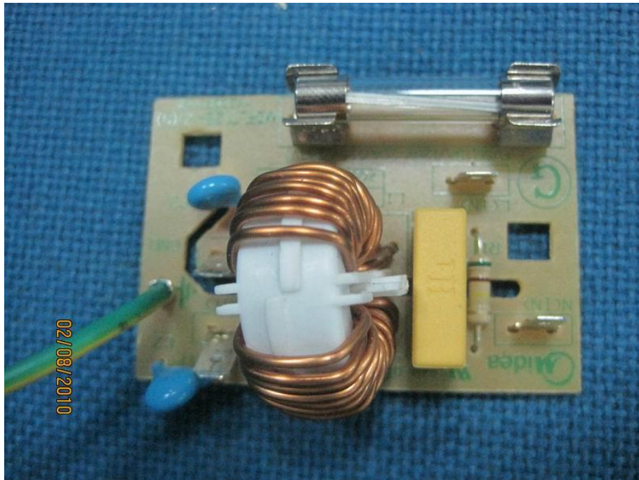
Power Filter Board Top View
