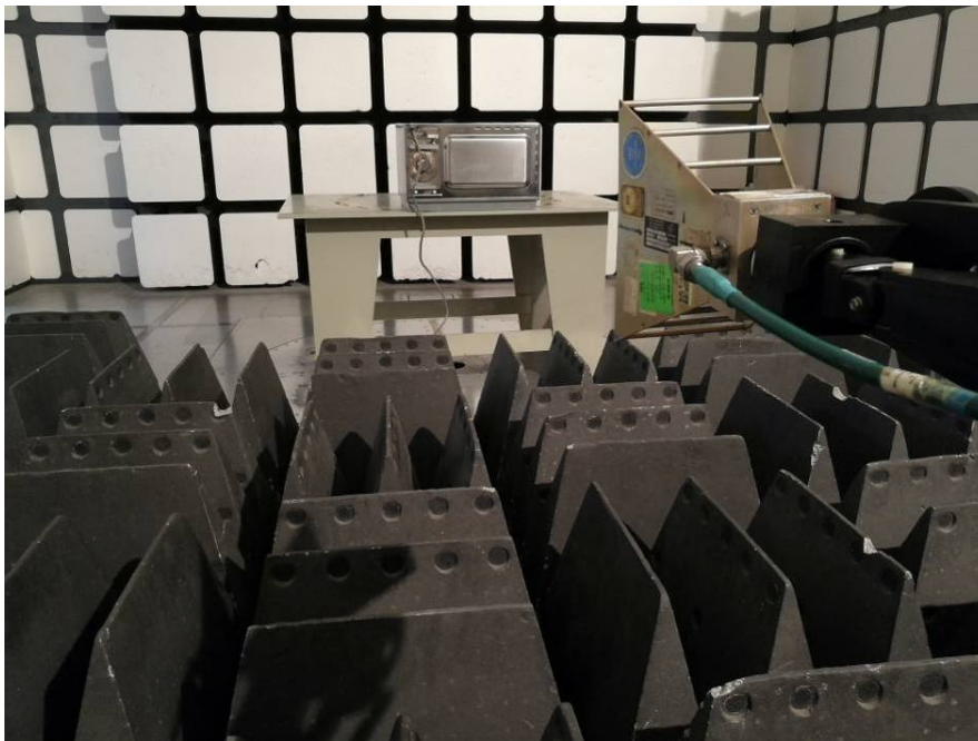
Radiated Emissions - Rear View (Above 1 GHz)
