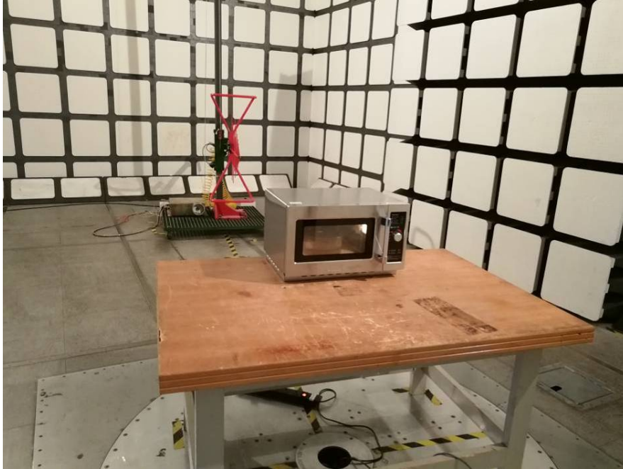
Radiated Emissions - Front View (30 MHz – 1 GHz)
