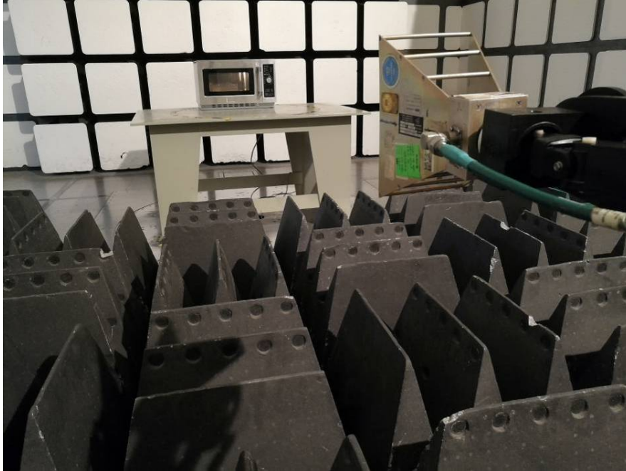
Radiated Emissions - Front View (Above 1 GHz)
