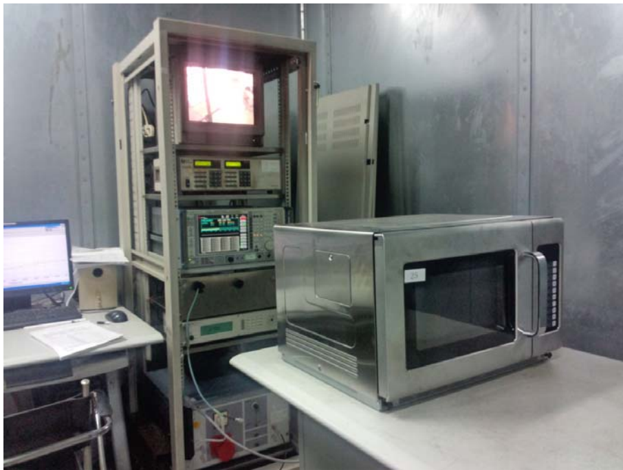
Conducted Emission Test Set-up
