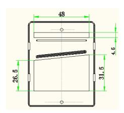
The New waveguide outlet opening
