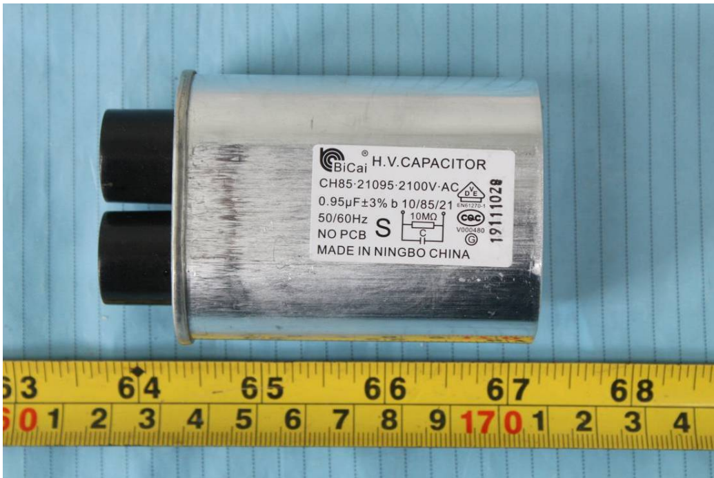
EUT – H.V. Capacitor View
