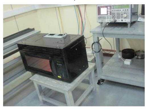
Radiated Emission Test Set-up (30 -1,000MHz):
