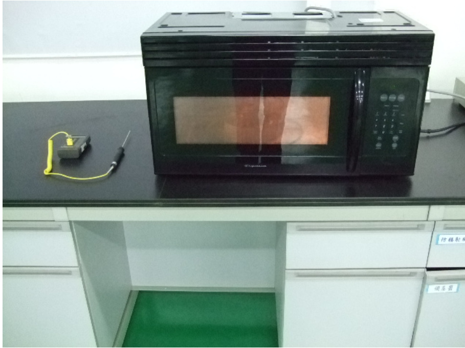
RF Output Power Test Set-up
