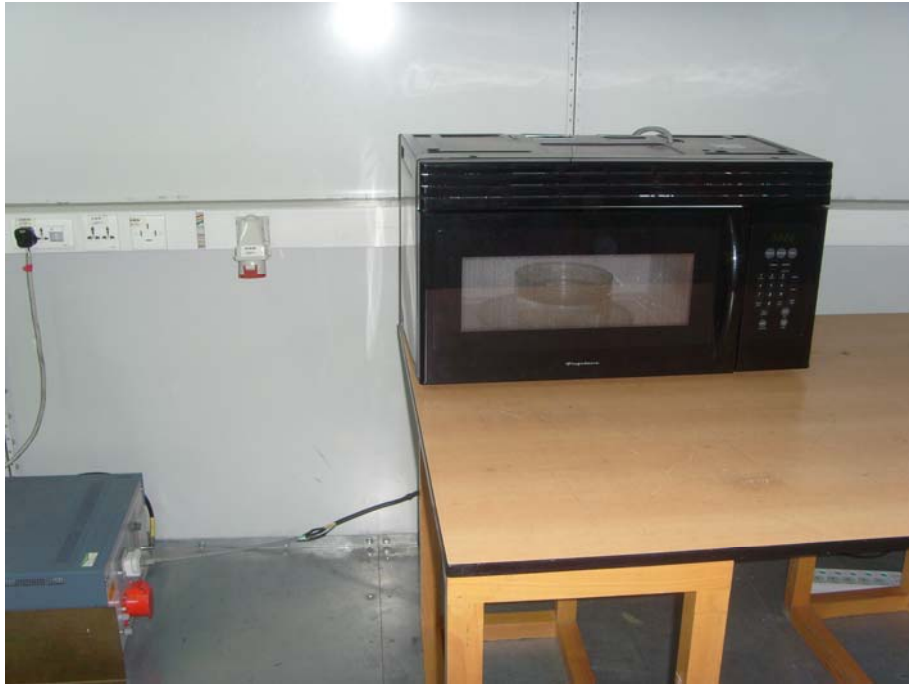
Conducted Emission Test Set-up
