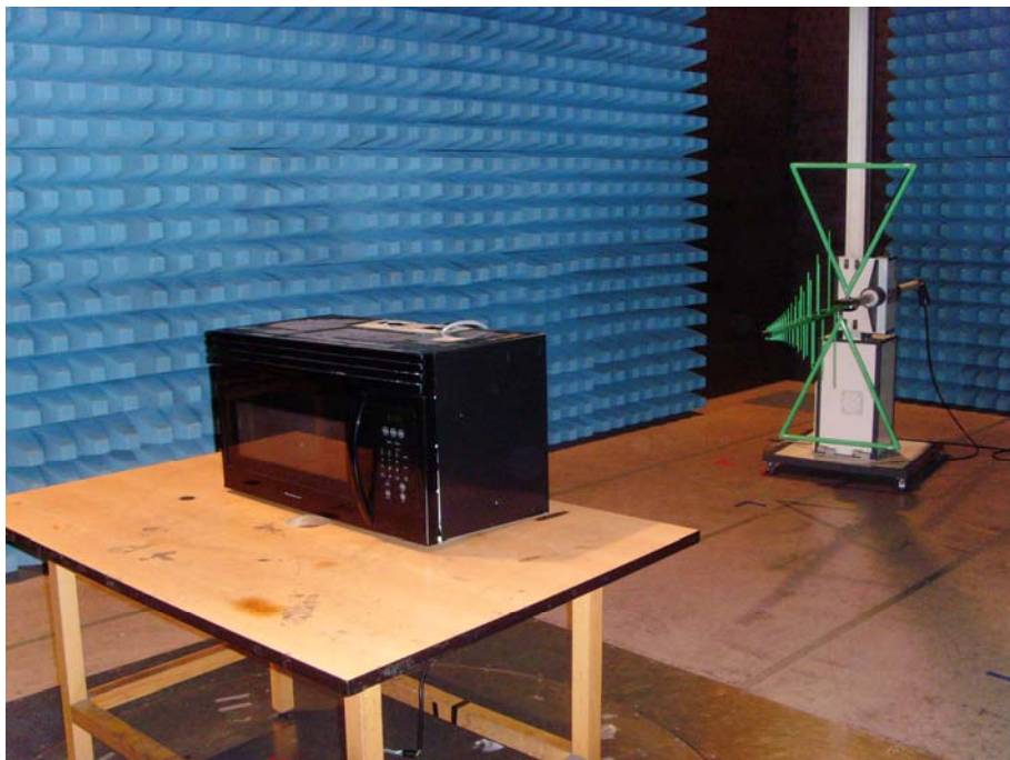
Radiated Emission Test Set-up (30~1000MHz)
