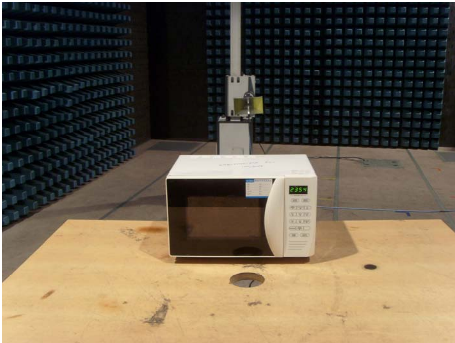
Radiated Emission Test Set-up (1~25GHz)
