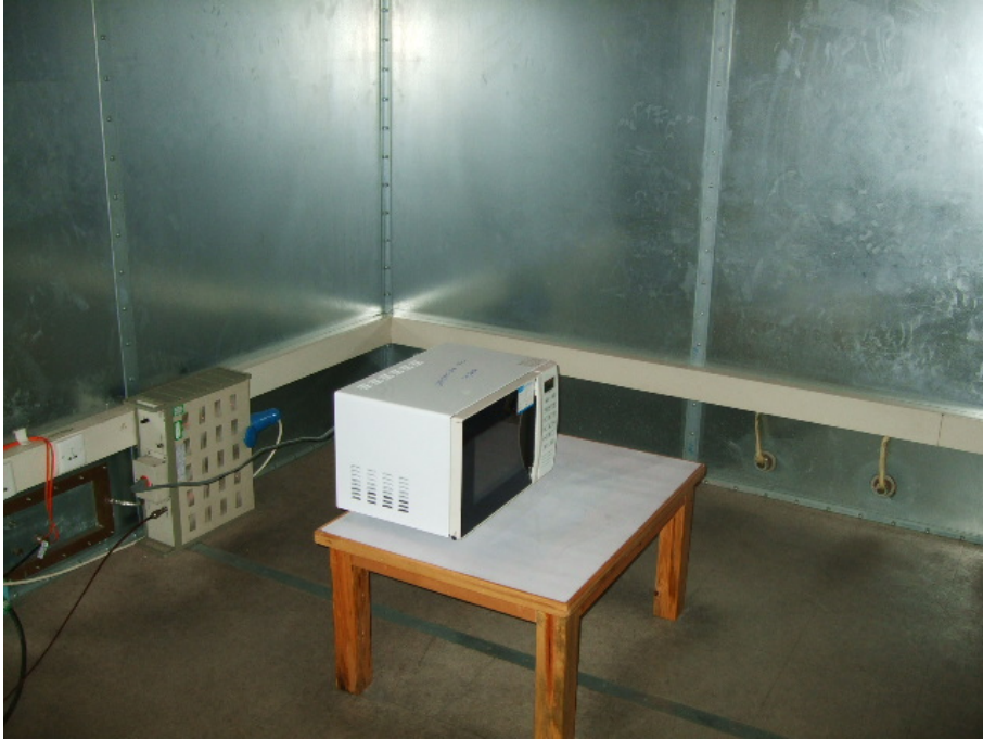
Conducted Emission Test Set-up
