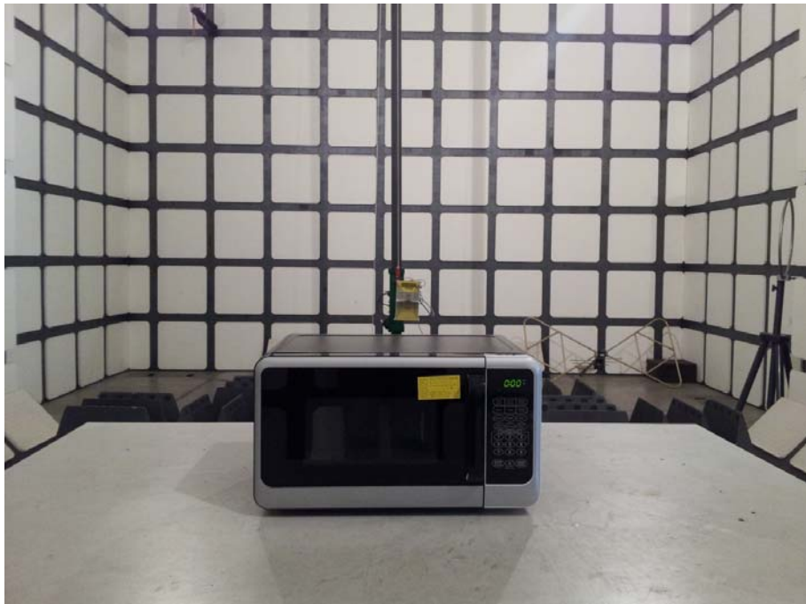
Operating Frequency Test Set-up
