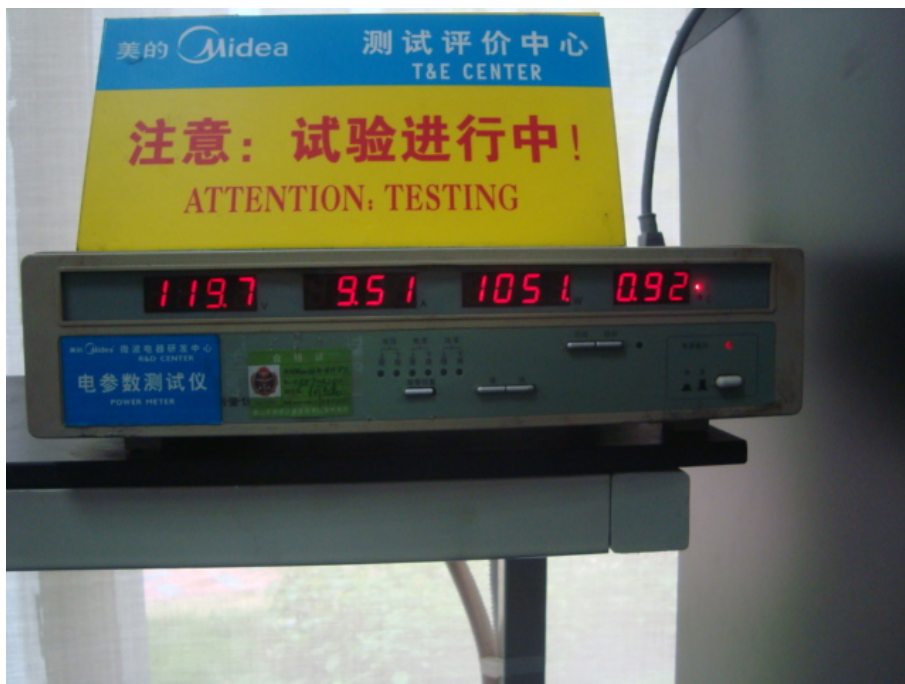
Input Power Test Set-Up
