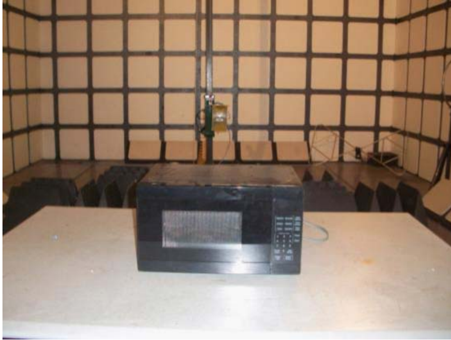
Operating Frequency Test Set-up
