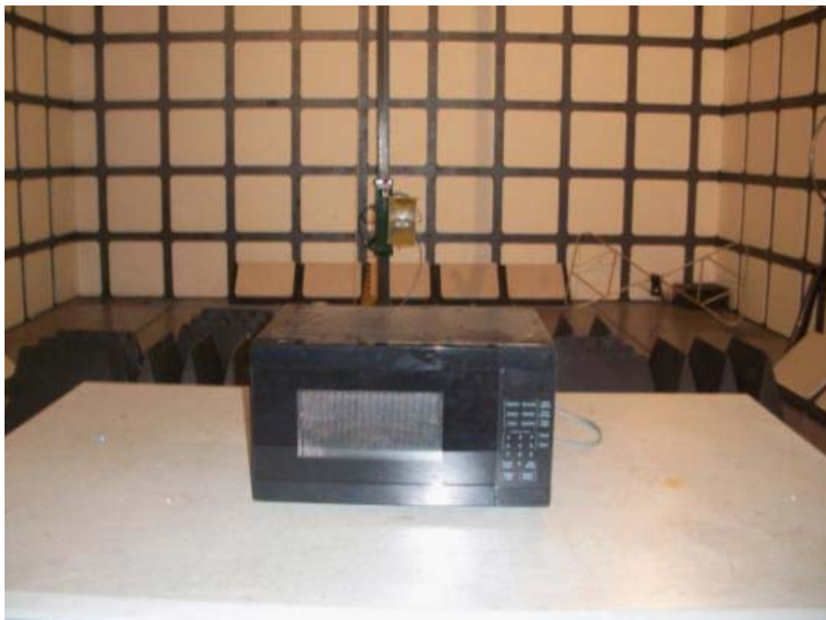
Radiated Emission Test Set-up (1-18GHz)
