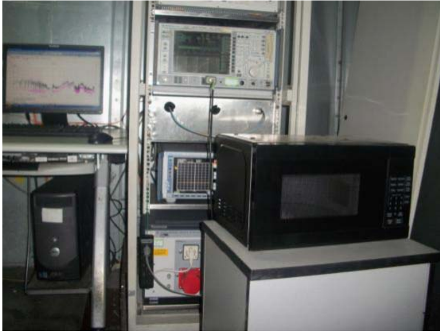
Conducted Emission Test Set-up
