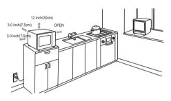
A minimum clearance of 3.0 inches (7.5cm) is required between the oven and any adjacent walls. One side must be open.
