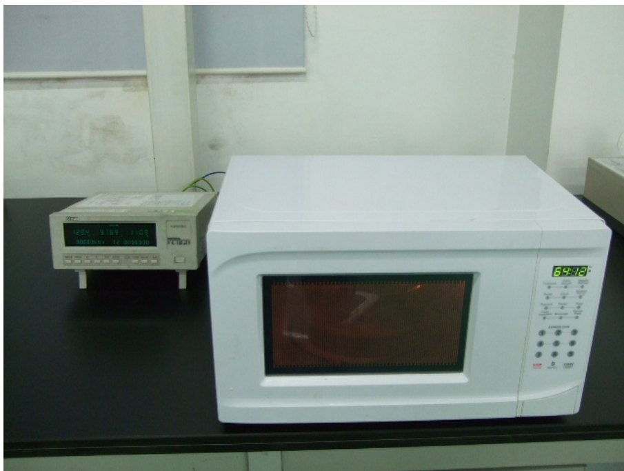
Input Power Test Set-up
