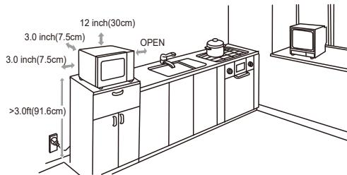
A minimum clearance of 3.0 inches (7.5cm) is required between the oven and any adjacent walls. One side must be open. The minimum installation height is 3.0ft(91.6cm).
