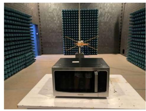
1. Radiated Emission Measurement below 1GHz
