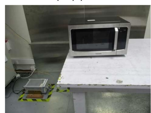
3. Conducted emission at AC mains input/output port Measurement
