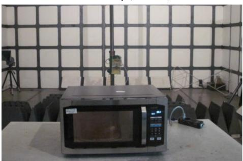
Radiated Emission Test Set-up (1-25GHz):
