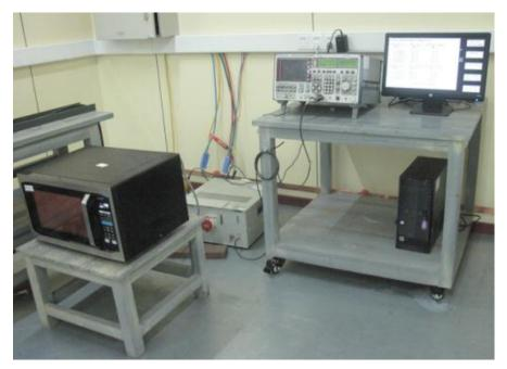
Radiated Emission Test Set-up (30 -1,000MHz):
