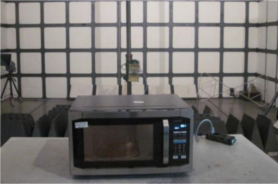
Operating Frequency Test Set-up
