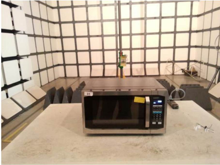
Operating Frequency Test Set-up
