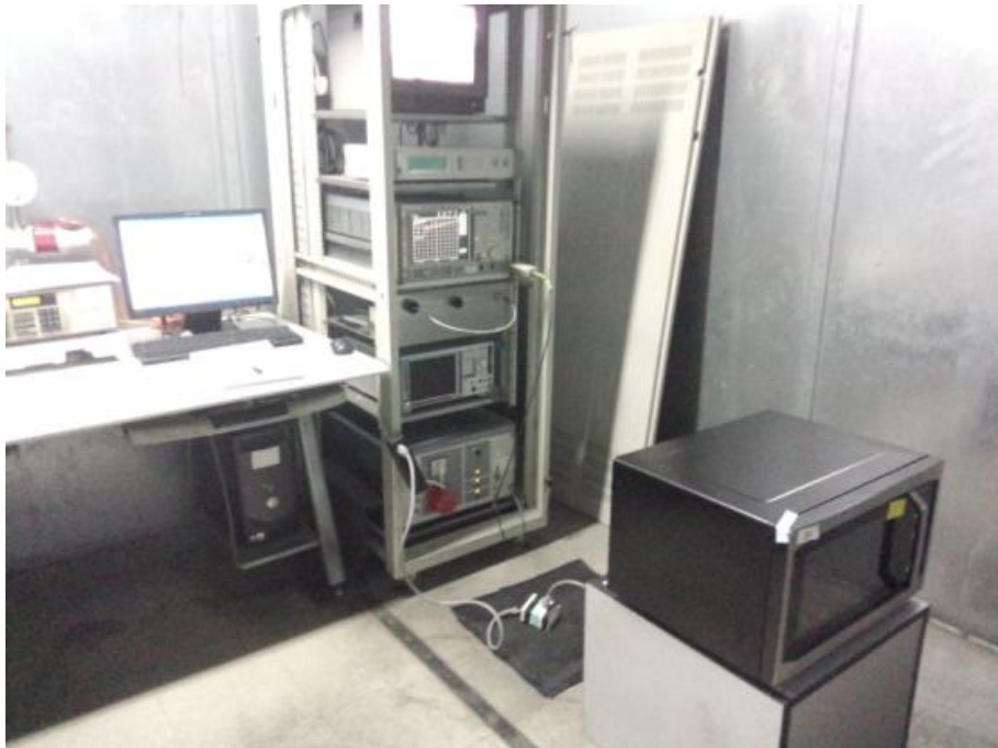
Conducted Emission Test Set-up
