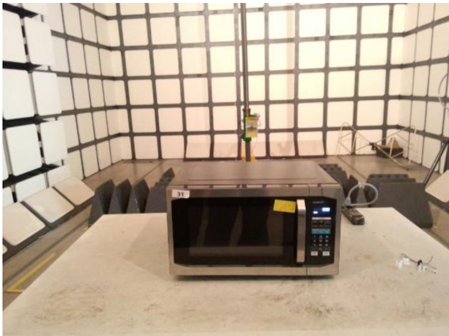
Radiated Emission Test Set-up (1-18GHz)
